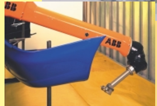
1. Single spray gun model mounts directly to robots.
